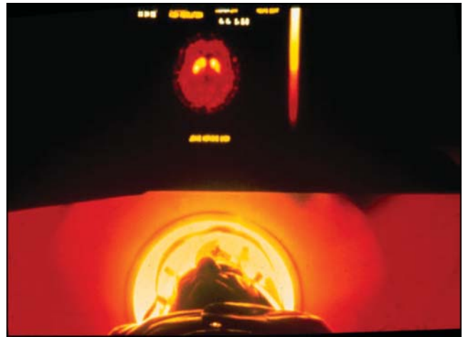
FIGURE 15. Very early dopamine PET images, such as this 1983 photograph of apparatus and resulting image, showed evidence of accumulation of tracers in the striatum but no separation of the caudate nucleus from the putamen.
